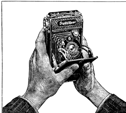
Fig. 8. Closing the baseboard
